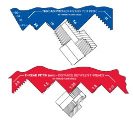
Line up threads along side the thread gauges until closest match is found. This section of the tool is unable to gauge female threads, however the corresponding male assembled with the given female can be used to identify the female thread pitch.
